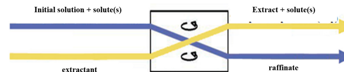
Figure 1 – The mechanism of the extraction process
